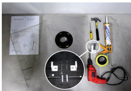
2. The tools required for installation are: Drill, hammer, screwdriver, glue for glass, Triangular rule ...
